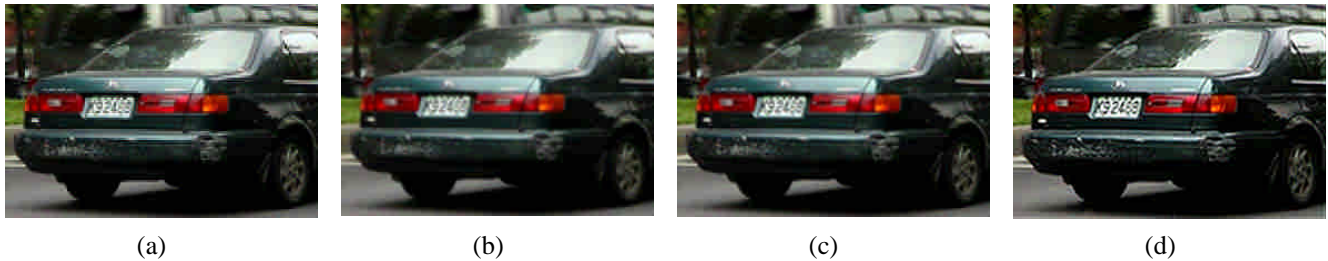
Figure 6: Reconstructed high resolution image from real LR images with multiple moving objects. (a) Image expanded by the zero-order interpolation method. (b) Image expanded by the bilinear interpolation method. (c) Image expanded by the bicubic interpolation method. (d) Image expanded by the proposed super-resolution method.
